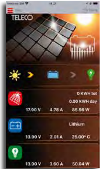
TELECO app with notification of low battery alarm, compatible with MPPT 20 1/B and 30/1B
